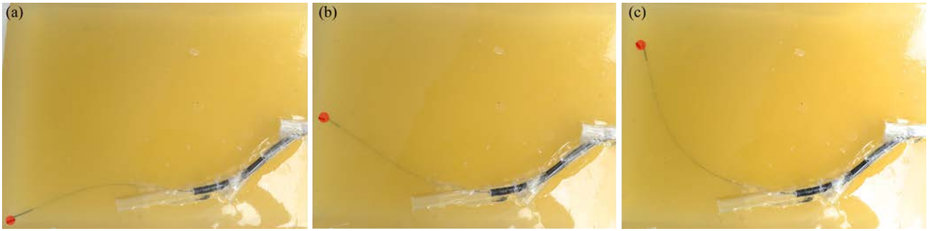
Fig. 7: The three-stage steering system deployed to three separate targets in the phantom. The tip error for each of the three runs was (a) 1.3 mm, (b) 0.5 mm, and (c) 0.2 mm.
