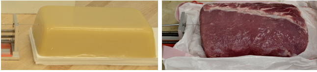
Fig. 6. (Left) Sim-Test tissue phantom. (Right) Porcine tissue ex vivo.
