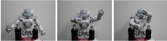
Fig. 6. The Nao robot uses a low-power Intel Atom CPU to solve a 10 DOF motion planning problem (from [26]) that avoids obstacles in order to drop an effervescent tablet into a glass while not spilling in the process.
